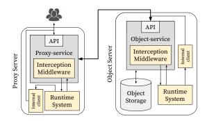
Fig. 3. High level architecture overview on OpenStack Swift
